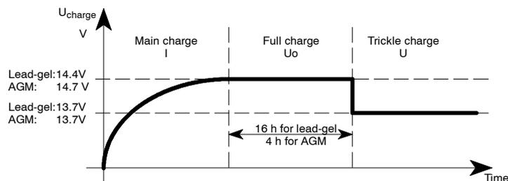
Fig. 3 Charging voltage curve with electroblock EBL 30
